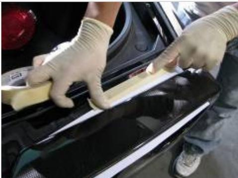
10. Use strips of masking tape to secure the perimeters of both paper templates to the vehicle.
