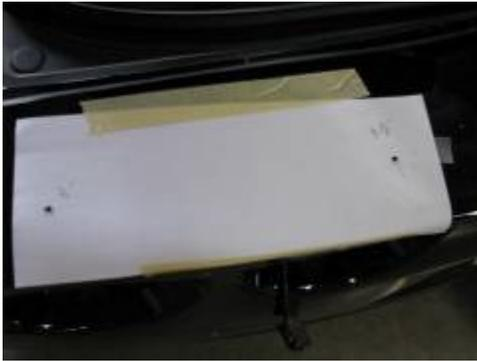
11. Remove the spoiler from the vehicle. Make sure the paper templates remain attached to the vehicle.
