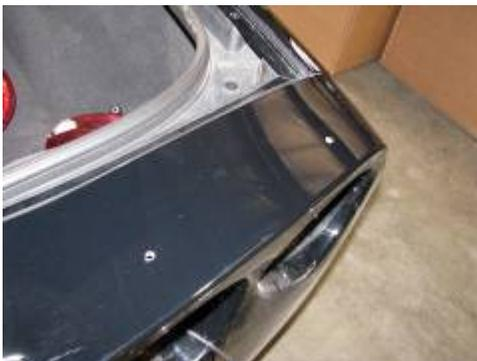
13. Drill 1/4" holes into the vehicle through the holes on the paper templates.
