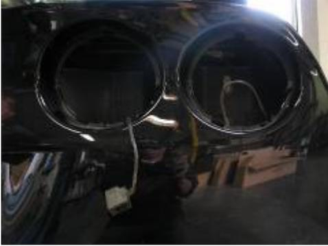
1. Remove the rear tail lights. There is 1 hex screw to remove near the top of each tail light.
