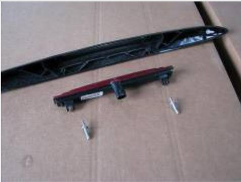
3. Disassemble the factory spoiler / brake light assembly.
