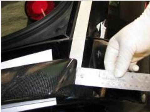
9. Align the spoiler to the vehicle. The spoiler should be centered and line up with the rear edge of the rear bumper cover. To help with centering, attach a strip of masking tape along the inner edge of the rear fender, extend the tape to the spoiler, then take measurements on both sides of the spoiler.
