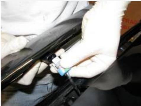
15. Plug in the rear brake light connector, then attach the rear spoiler to the vehicle using the hardware that was set aside earlier. (2 of the factory holes will be re-used)
