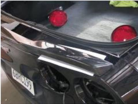
8. Place the new spoiler onto the vehicle.
