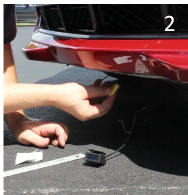
Wipe 3M promoter for sensor & wire clips mount.
