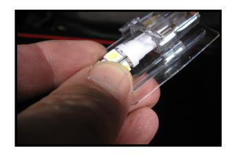
Using a flat blade screwdriver, carefully pry the footwell light housing out of the panel. Remove the factory bulb. DO NOT USE METAL OBJECTS TO REMOVE BULB TO AVOID BLOWING FUSE. Bulb may be hot.
