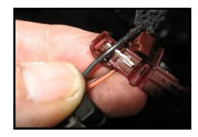
Using the supplied quick tap, Place the gray wire in the metal clip then close the connector . You may have to use pliers to make sure it latches. Plug the red wire from the led harness into the back of this connector and press firmly until it seats. It will be tight. See next picture.
