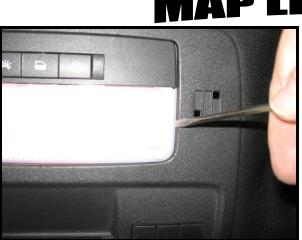
Using a small flat screwdriver, gently pry the map light lens from the housing.
