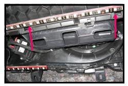
Center the light bar on the rib that goes across the bottom of the panel under the glove box door. Open the glove box door to be sure it doesn't hit the light bar. Peel and stick the light bar. You can also drill holes in the ribs and attach with wire ties.
