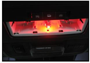
Plug the led bulb into the factory position. Leds are polarity sensitive so if it doesn't light, turn it 180 degrees and re-install. Make sure the interior lights haven't timed out. Re-install the map light lense. That's it!!
