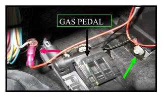
Red arrow shows positive wire fully seated in connector. Green arrow shows bolt for the ground wire. Remove bolt with a 10mm wrench, install ground wire and reinstall bolt. Lights should now work with the interior lights. Be sure lights havent "timed out". Secure all wires away from gas and brake pedal. That's it!
