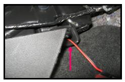
On the passenger side the red arrow shows a bracket that may get in the way. You can pass the light bar through the hole in the bracket or go around the bracket..
