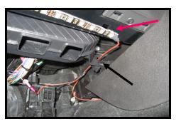
Pass the flexible drivers side led strip through this area (black arrow). After wiping mounting area with alcohol swab, attach led strip to panel under drivers area. (red arrow). If it doesn't stick well, rough up the mounting area with sandpaper or emery cloth, wipe with alcohol and attach strip.
