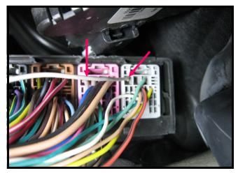
Look above the gas pedal for the module shown. The red arrow shows the gray wire in the gray plug that must be tapped into for the positive wire. There is a latch on the bracket you can push to pull the module down a little for easier access. Carefully cut one or two of the tie straps to make it easier to access this gray wire. Test with a test light to be sure you have the correct wire. Test light should mimick the dome light.
