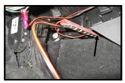
From the drivers side, pass solid led bar through the front of the console area to the passenger side. There is a open area above the carpet in front of the console.
