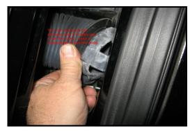
Pulling the door boot back will help in fishing the wires through to the footwell area.
