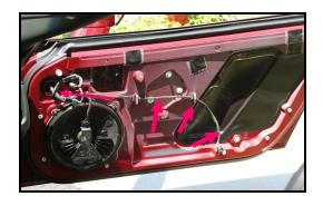
Route the wire out of the inner door panel and up to the main wiring plug near the front upper part of the door. (long arrow). Using a pic or awl poke a hole in the rubber boot and pass the wires through into the tube between the door and the body. Using a wire hangar fish the wire through the door boot to the footwell area.
