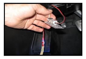
Using the supplied scotch lock connectors, tap into the factory footwell light wires. Align red to orange and black to white. Lights should now operate. Make sure the lights havent "timed out" which the car will do after about 15 minutes.
