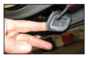
To start installing the puddle strips, locate this plug at the bottom front of the doors. Using a small pic or awl, make a hole just large enough for the wires. Silicone opening to make watertight. Position strips where you want, wipe area with provided alcohol pads, peel and stick the strips in place.
