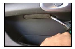
The driver's door has a total of two bolts. They are located right below the door handle. If you look closely, you will see a small plastic cover. Remove the cover and you will see the two bolts. Remove the 2 bolts.
