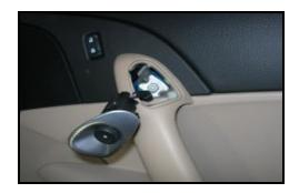
On the passenger side Pry the door button out with a small screwdriver. This will allow acess to one of the secrews.
