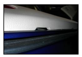
With the second screw removed you can start removing the door panels from the clips that hold it in place. Locate the indentation on the bottom center of the door panel to the right of the reflector. Using the panel removal tool, start here to pry the panel off. Use a shop rag to protect the paint. It will require some force and you will hear a lot of noise as the clips disengage from the door. There are 8 clips to disengage
