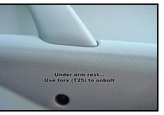
The second screw on the passenger side is below the handle.
