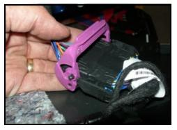
After releasing all the panel clips you must unplug the wiring harness by releasing this purple clip. Unplug the harness and set the panels aside.
