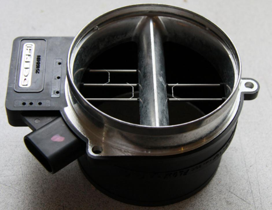
Place the Halltech HC.125 Honeycomb into the MAF. Be very careful of sharp edges from the Flow Jet cutter. The aluminum edges can cut you.
