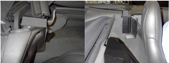
Insert the Vette Net legs into each pipe and gently tap on the top of the net to make sure it sets all the way down into the legs.
