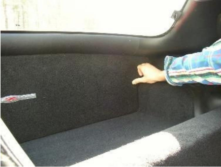
Lastly, do a quick push on both sides one more time just to make sure everything is snug and aligned. Push the bottom of the partition back into the car until it is vertical with the floor. Then go into the trunk and loosely attach the Velcro straps.
