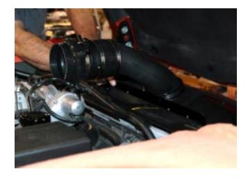
Slide airbox assembly into place as shown. Place remaining hose clamp over hump hose.
