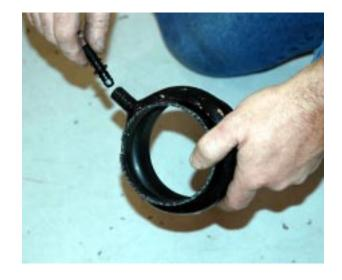
To install hump hose to MAF sensor, align cut out notch on hump hose with protrusion on MAF sensor.
