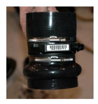
Attach supplied air inlet to other end of 4" hose with the nipple on the hump hose in the 10 o'clock position as shown.
