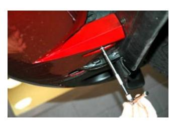
Remove (2) plastic push pins holding radiator shroud to bumper beam.
