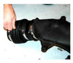
Remove black plastic nipple from stock bellows as shown.
