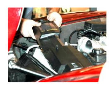
Disconnect electrical connector for under hood light.
