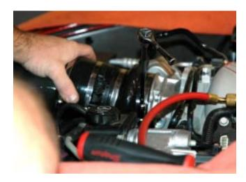
Use (4) of the supplied push fasteners to secure airbox flange to the shroud. Pinch pieces together as tight as possible when pushing in center of fastener to ensure a tight fit.
