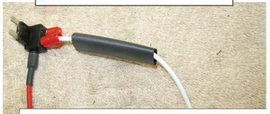
Slip back or carefully cut the shrink wrap that covers the fuse and spade. This will expose the 10A fuse and the tap at the end of the white wire. NOTE. color of shrink wrap and tap my be different than picture
