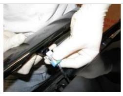
15. Plug in the rear brake light connector, then attach the rear spoiler to the vehicle using the hardware that was set aside earlier. (2 of the factory holes will be reused)
