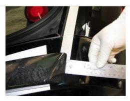
9. Align the spoiler to the vehicle. The spoiler should be centered and line up with the rear edge of the rear bumper cover. To help with centering, attach a strip of masking tape along the inner edge of the rear fender, extend the tape to the spoiler, then take measurements on both sides of the spoiler.
