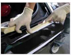
10. Use strips of masking tape to secure the perimeters of both paper templates to the vehicle.
