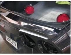
8. Place the new spoiler onto the vehicle.
