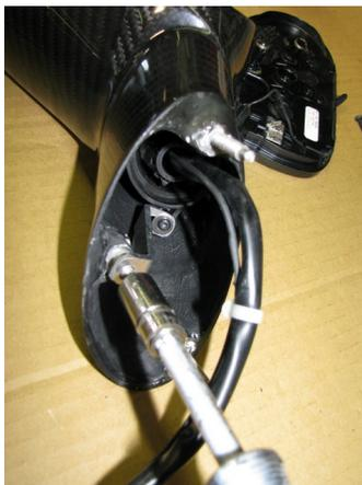
**Transfer internal parts to the new housing.**
