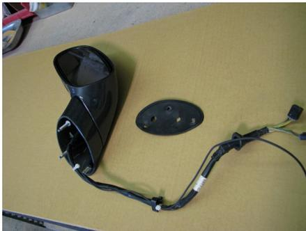
Remove the mirror assembly from the vehicle. The gasket will be re-used.
