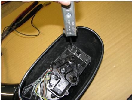
**Remove two small Torx screws. The new housing will have two new screws to replace these.**
