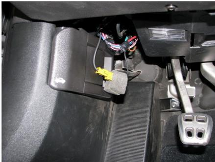
Find and unplug the yellow XM Radio connector (2006-Up with XM option)
