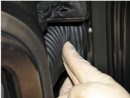
Feed wire through rubber tunnel.
