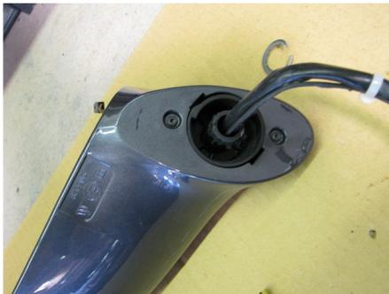
**Remove two screws at the bottom of the main housing. One of these screws will be re-used in the new housing.**
