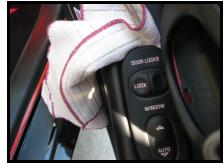
Now remove the passenger side panel by prying up on the TOP of the panel. Remove and unplug the panel and using the same procedure as before, install the 2 leds. Again, they are polarity sensitive so you may need to turn them 180 degrees if they don't light. Always keep in mind that the interior light may "time out" after about 15 minutes so you may need to re-activate the interior lights. Re install both panels and enjoy the new lights!
