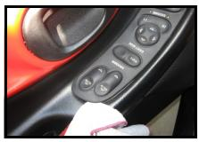
Remove the drivers window switch by prying up on the BOTTOM of the switch. Use a flat blade screwdriver and a shop towel to protect the panel and switch. Press the release tab and unplug the switch.
