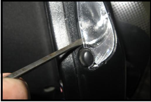
Begin by carefully prying out the map light lens with a small flat screwdriver. Best place to start is near the button.
