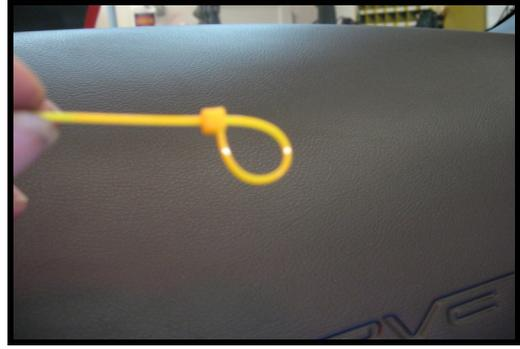
Remove the factory bulbs. (careful, they may still be hot). A little trick we like to use is using a small plastic wire tie to slip around the base of the bulb, pull it tight and pull the bulb out. Avoid using anything metal to remove them as you may short out the contacts.
