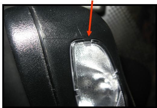
Re-install the lenses by first engaging the tab (red arrow). Then press the lens back into place. Repeat this procedure for both map lights. That's it! Enjoy the new lights!
