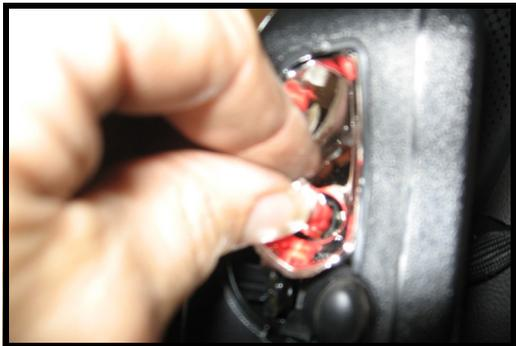
Insert the new led bulb. It is polarity sensitive so if it doesn't light, turn it 180 degrees and insert it. Make sure the interior lights haven't "timed out" which they may do after about 15 minutes.
