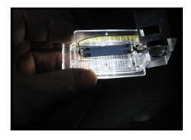
Un-hook the 2 wire loops from the end on the factory bulbs. (careful, they may still be hot). Remove the bulbs. Install the new led bulbs and test. Led bulbs are polarity sensitive so if they don't light, swap ends and re-test. Be sure to face the leds toward the clear lens and not toward the metal shield. Make sure interior lights havent timed out which they may do after about 15 minutes.
