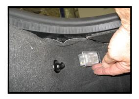
Remove the rear compartment lamps from the carpet.
