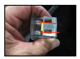
Remove the bulb shield by un-latching it from these 2 plastic tabs.
