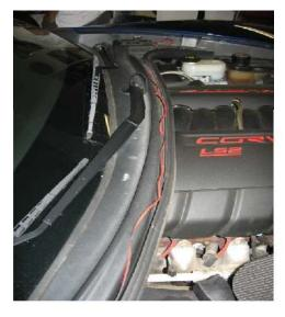
String long led wire across the cowl. Remove cowl weatherstrip. Using electrical tape, secure wire to the cowl and replace the weatherstrip to conceal the wiring.
