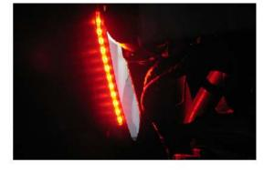
Drivers side led strip attached to inner side of fender facing the shield area. Reinstall shields if removed. Helpful Hint: Lift edges of adhesive pads before installing shields so you can easily grab and remove backing.
