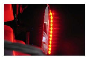
Clean mounting area with alcohol. Position led strip centered in cove opening and attach. Attaches to inner side of fender behind the lip.
