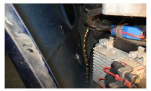
Route pass. side leds behind battery and drop into the cove area.
