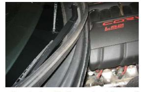
This shows the wire taped to the cowl and the weatherstrip going back in place.
