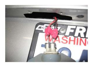
Use the 2 supplied scotch lock connectors to connect the led wires, black to black and brown to red. Test the lights to make sure your connections are good.
