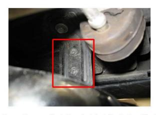
This shows the rear facia bracket that the leds will attach to on the back side between the screws you see inside the red box. Center the led bar between the brackets, peel and stick the led bar to the backside of the brackets.
