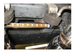
This picture shows the location of the exhaust leds. Leds are attached to the rear of the rear facia brackets facing the front of the vehicle, Note the routing of the wires up towards the license plate lights. This is where the coat hangar comes in handy.
