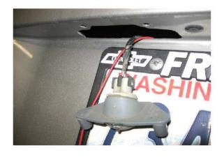
Remove the 2 screws that hold one of the license plate lights on. Route the led wires as shown. Make sure the wires are clear of all exhaust pipes so they dont get burnt.
