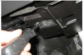
Using a flat blade screwdriver, pry at the center of the factory light and remove it from the panel above the footwells.
