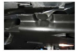
Locate the 2 retainers that hold the panel in place. Using a forked panel removal tool or equivilent, pry the retainers out and drop the panel down for access.
