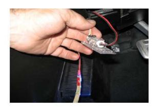
aligning the red wire with the orange wire in the socket. Black aligns with white. Make sure lights are now lit. Make sure lights havent "timed out". Fold wires back and re-install light housing.
