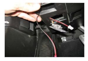
Route the connector of the leds down from the top of the Push the connector into the socket where the bulb was panel and through the hole where the light housing installs.
