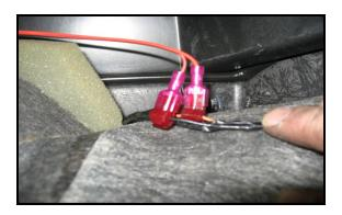
Using the supplied connectors, tap into the factory wires. Fold and crimp connectors using pliers, then plug led wires into the back of the connectors you just installed. Connect red to orange and black to black. If the leds don't light, check all connections and make sure the lights have not timed out after about 15 minutes. Re-assemble all panels and enjoy the new lights!
