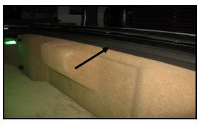
On C5 convertibles: Front edge of the weather strip pointing forward into the trunk. The C5 coupes, C6 convertibles and C6 coupes use this same mounting area. Be sure to clean weather strip with alcohol swabs as armour all may have been applied.
