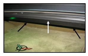
This shows 2 areas on the c5 convertible. Bottom of the large square brace (black arrows). Between the trunk weather strip and the square brace (white arrow) They can also be applied as in the next picture..
