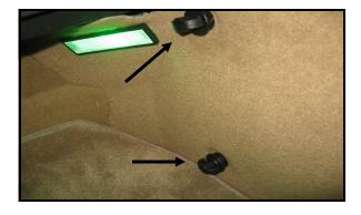
Remove 2 cargo net nuts and light to gain access to wiring behind carpet panels. Route wires from led strip behind panels on either side to area near the factory lights.
