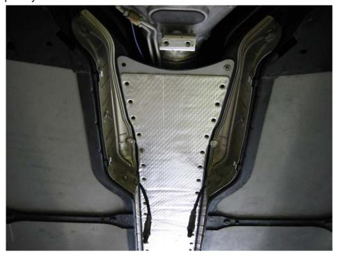
Don't force a screw in if it feels as if there is an unusual amount of resistance. A drop of Tap Magic or machine oil might help to thread it in more easily. Push the plate up against the frame rails to relieve tension on the screws as you turn them in by hand. Turn them in evenly as you go to avoid binding one side relative to the other. Once they have all seated by hand, you're cleared to torque them.
