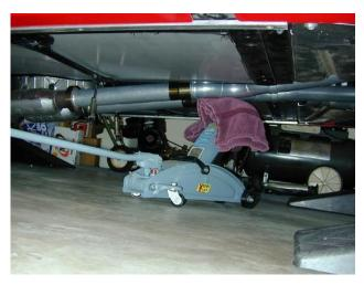
Below is a shot of the stock H-pipe and center exhaust section removed. At the very top bottom of the picture, you can also see the flanges of the exhaust manifolds. Remember, the exhaust manifolds do not need to be removed for the installation of Elite's Tunnel Plate. You can also see the location of the O2 sensors and mounting brackets.
