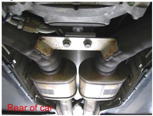
At this point you can place a jack as best as you can under the center of gravity of the exhaust. Holding the exhaust steady, unscrew the spring hanger bolts and the front exhaust mounting bracket screws completely and slowly lower the exhast down and maneuver out from under the car. Once again, make sure you're careful to clear the O2 sensors and other structures.
