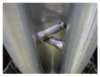
Next, you will need to remove the (6) bolts from the driver's side and passenger side Header 3-bolt Tri-Flange shown below. These bolts may need a little extra effort to loosen.
