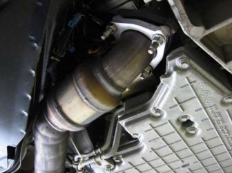
This view below, from the rear of the car, shows the (2) sets of muffler bolts that need to be removed.
