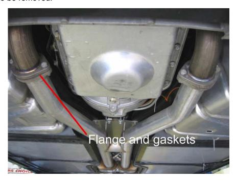
Next, use a 13 mm socket and wrench to loosen, but don't remove yet, the (2) spring hanger bracket bolts pictured below. Don't remove them yet. You'll want to leave these until last so that the exhaust stays in place until you're ready to lower it. Remove the bolts on the front and rear flanges that connect the h-pipe (or x-pipe) to the exhaust manifolds and to the catback over-axle pipes.
