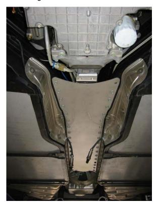
The stock plate is held in place by (36) 6x1.25 mm bolts. To remove the stock plate, use an 8 mm socket on a 6-inch extension to first loosen, but not remove, two of the center-most screws, one on each side opposite each other. Then completely remove the other 34 screws. See the picture below. Finally, remove the two you first loosened while supporting the plate to prevent it from falling. Then carefully move the plate away from the car.
