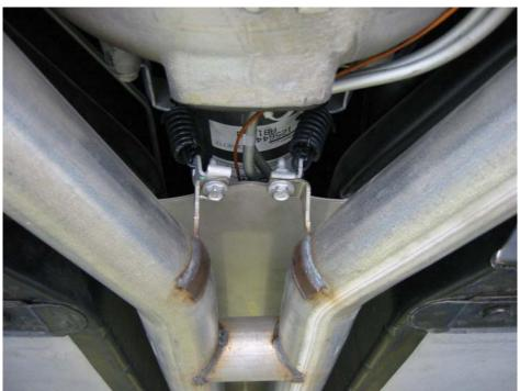
If your exhaust has the stock h-pipe, you'll need to also loosen the two front exhaust mounting bracket bolts using a 13 mm socket (see below). Do not remove them at this time. Leave them attached to help support the exhaust. The h-pipe should now be hanging loosely by these two front bracket bolts and the spring hangers.
