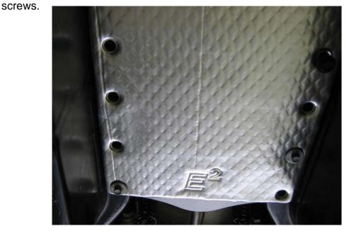
Start the rest of the screws and then carefully **hand-tighten** them using the 6-inch extension with the 8-mm socket. Snug them all down sequentially until they are completely seated.
