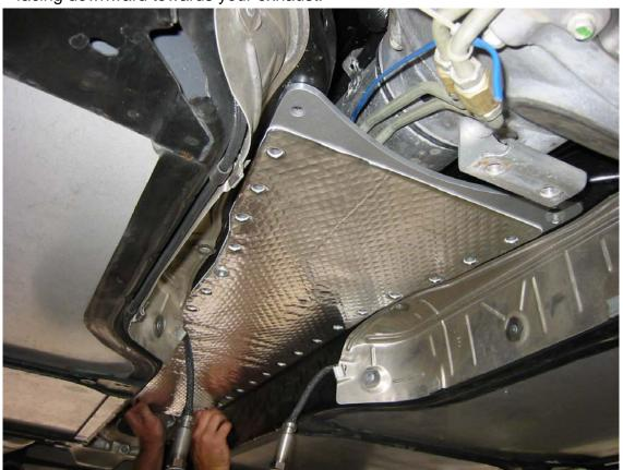
You should be able to read the E² logo from underneath and it should be at the rear of the tunnel. Carefully lift it into place and start two of the screws on opposite sides near the center of the plate to hold it in position and to bear its weight. You WILL reuse the original (36) screws that we removed during the first section. Even with the 3/8" thick plate, there is plenty of thread left in the original
