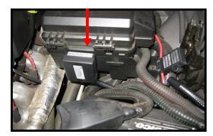
After all wires are secured and lights are working, You can now mount the control box. The box is not water-proof so cover when washing engine compartment. You can now re-assemble all shields. Remember, the Inner fender panels have a hooked clip on the top that should go in first. Enjoy the new lights!!
