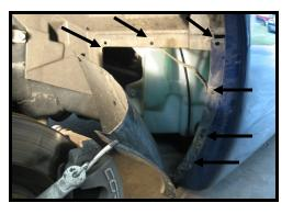
There are 2 styles of inner fender shields depending on the year and model of c6. This shows 1 style. Remove plastic retainers so you can pull shield back to gain access to cove area.
