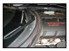
Place the remote control box by the battery and stretch the long led wire across the cowl. Pull the cowl weather strip off by pulling forward on it.
