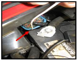
On the passenger side, Use a coat hangar to find a path down to the cove area. Route leds down to the cove opening and use the same procedure to mount them as the drivers side.
