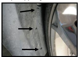
On GS and other later model c6's this is the style of inner fender panel. Remove 3 plastic retainers by pulling the center pin then remove the entire retainer. There is also a 8mm bolt on the bottom you can remove. Your not done yet, there are 5 clips that hold the panel to the outer lip of the fender.
