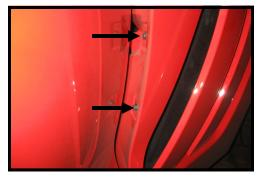
If you plan on removing the cove shields to paint, you need to remove these 2 screws from the rear of the fender. Open door, put protective tape around this area to protect the paint. The shield is also held on by 2 adhesive pads. New adhesive pads provided.
