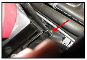
Below the battery tray along the frame rail there is a ground nut. Place the black wire from the control box over this stud and attach with the provided nut. You can now test the cove lights.
