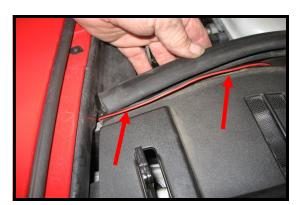
Secure the wire across the cowl by inserting it into the weatherstrip and pressing the strip back in place across the cowl area.
