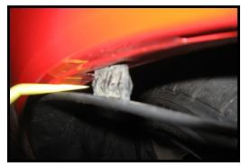
Using a panel removal tool and a shop rag to protect paint, pry between the panel and fender to unlatch these clips. The one at the top of the fender has a hooked retainer so remove the 2nd and 3rd ones first
