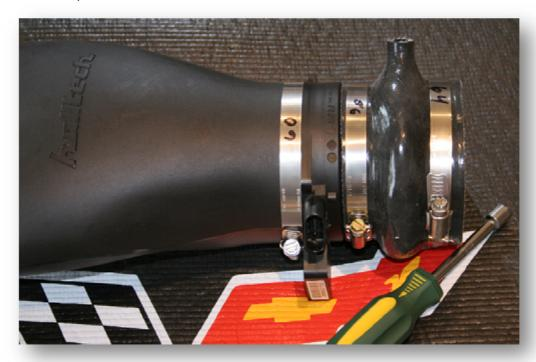
4) Check the filter carefully for any loose rubber that might have dislodged during shipping, and then set it down in the bottom of the shroud area. Install the bridge assembly to the throttle body, tighten the hose clamp, and insert into the filter. DO NOT OVERTIGHTEN!
